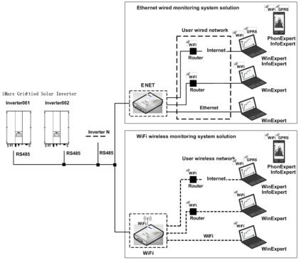
Figure 34 Monitoring system of inverter
