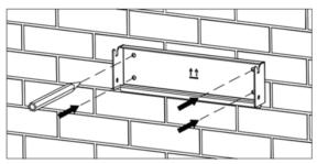
Figure 10 Determine the punch position
