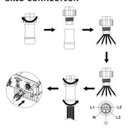
Figure 19 AC connection of single-phase inverter
