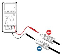
Figure 18 DC input voltage measuring
