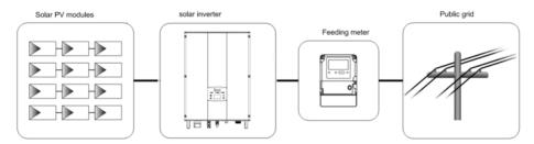
Figure 1 Application of the series grid-tied solar inverters
