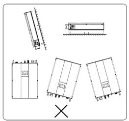
Figure 9 Installation position
