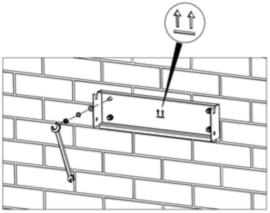
Figure 13 Fix the installation bracket
