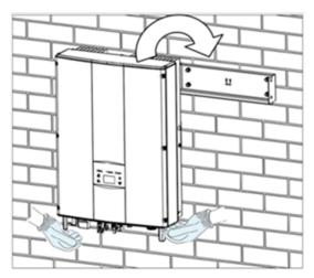
(5) Hang the inverter onto the installation bracket and ensure the installation is firm enough. As shown in Figure 14.
