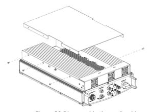
Figure 20 Disassemble the cooling bin
