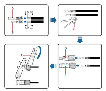
Figure 17 MC4 DC connector and PV string connection
