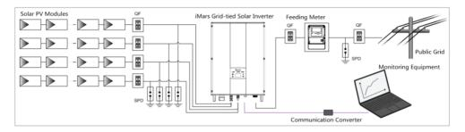
Figure 16 PV grid-connected system diagram
