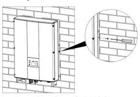
Figure 15 Installation of M5X20 bolts
