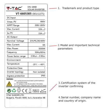
Figure 4 Inverter nameplate
